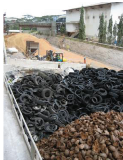
Pic.2: Coconut shells, Tyres, Wood chips and Rice Husks as alternative Fuel in a cement Plant
